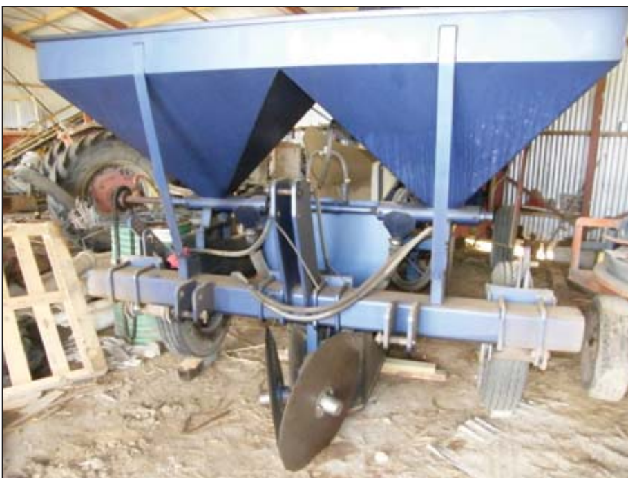
A wide chute disc opener built by Hodge Industries and connected to the old billet planter.
