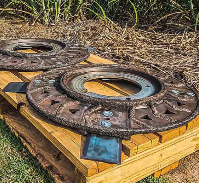
Comparison wear on the end of the blade when using a standard base cutter disc (A) versus the new self-sharpening EHS base cutter disc (B).
