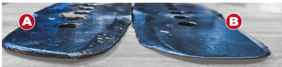
Comparison wear on the end of the blade when using a standard base cutter disc (A) versus the new self-sharpening EHS base cutter disc (B).
