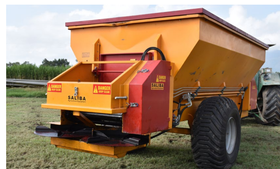
Pictured: The Saliba spreader, designed to spread material in a band from the front as well as broadcast material out the back, allows Herbert grower Allan Pace to apply low rates of mill ash or mill mud at a cost effective rate
