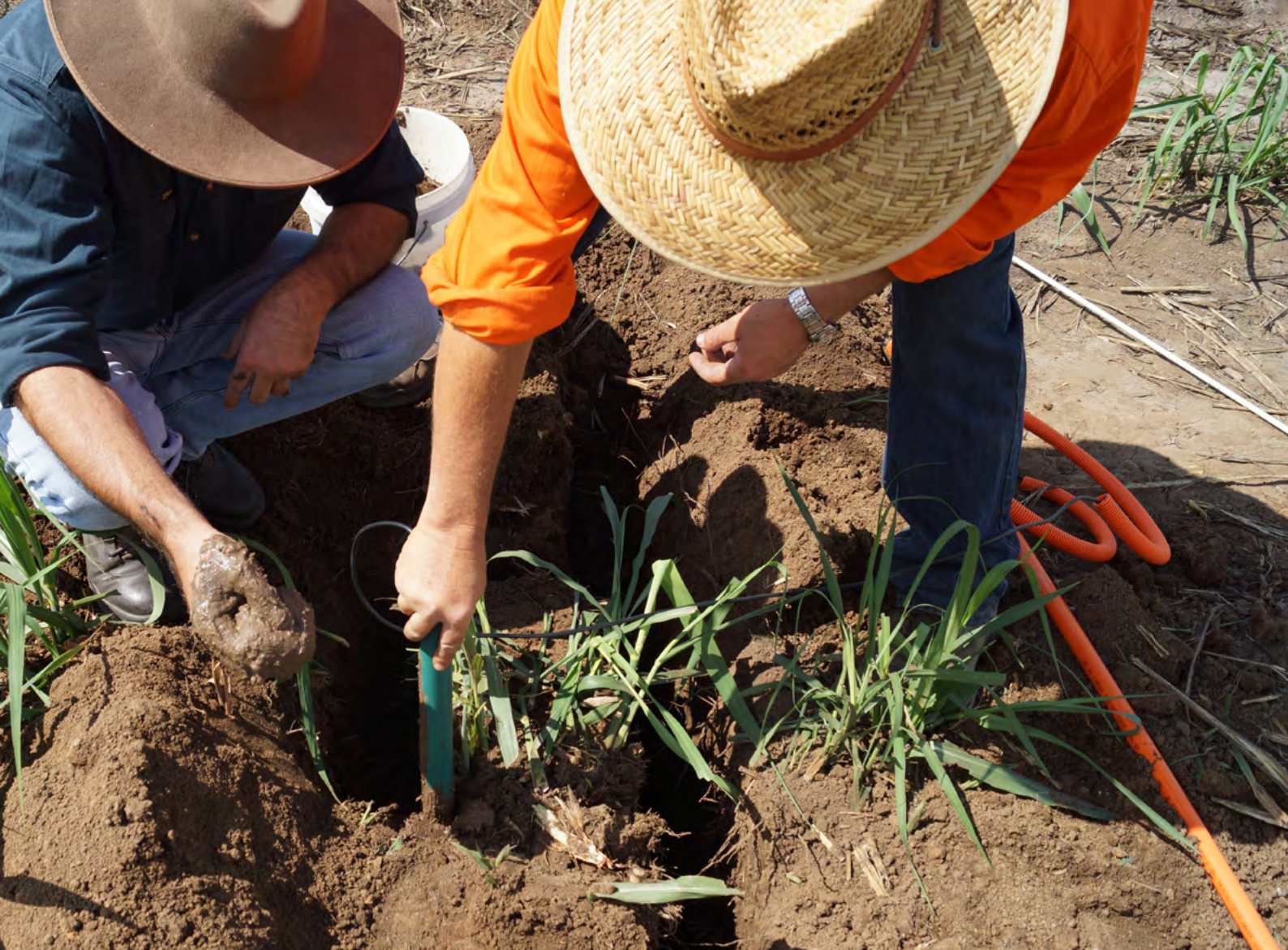
Pictured: Agritech Solutions' Steve Attard and Michael Hewitt install a soil moisture probe on a Burdekin cane farm as part of the region's soil moisture monitoring program.
