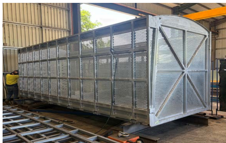
Redesigned road freight bin under construction in Gympie, 3 bins per B Double
